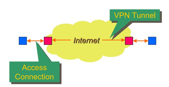
AC can be physical PPP or Ethernet link, FR or ATM VC, VLAN, MPLS LSP, etc.
